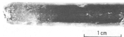
Figure 1 Single crystal of \text{Co}_{0.525}\text{Fe}_{0.475}\text{TiO}_3 grown by the floating-zone method.
